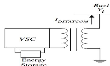
Figure (1) an example of STATCOM connected to the bus i [8]
