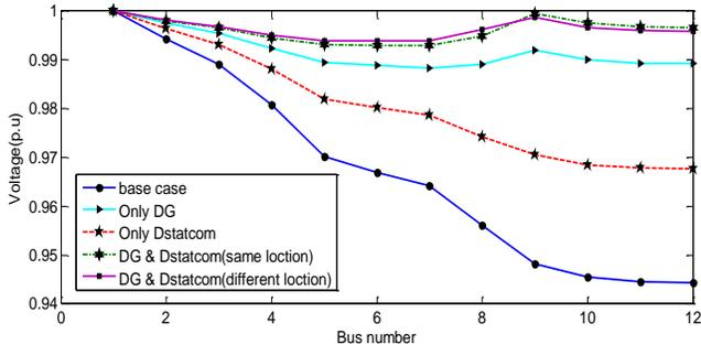
Figure (7) Voltage profile curve in five states in 12-bus network
