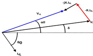
Figure (3) Voltage and current phasor diagram of the system shown in Figure (2) [8]
