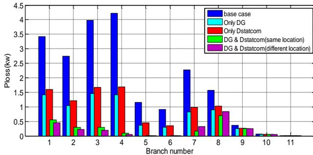
Figure (8) losses reduction curve in five states in 12-bus network
