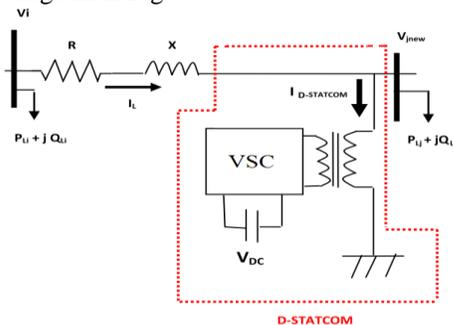
Figure (4) installing STATCOM on J bus in proposed distribution network [8]
