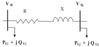
Figure (2) Single-line diagram of two consecutive load buses in distribution network
